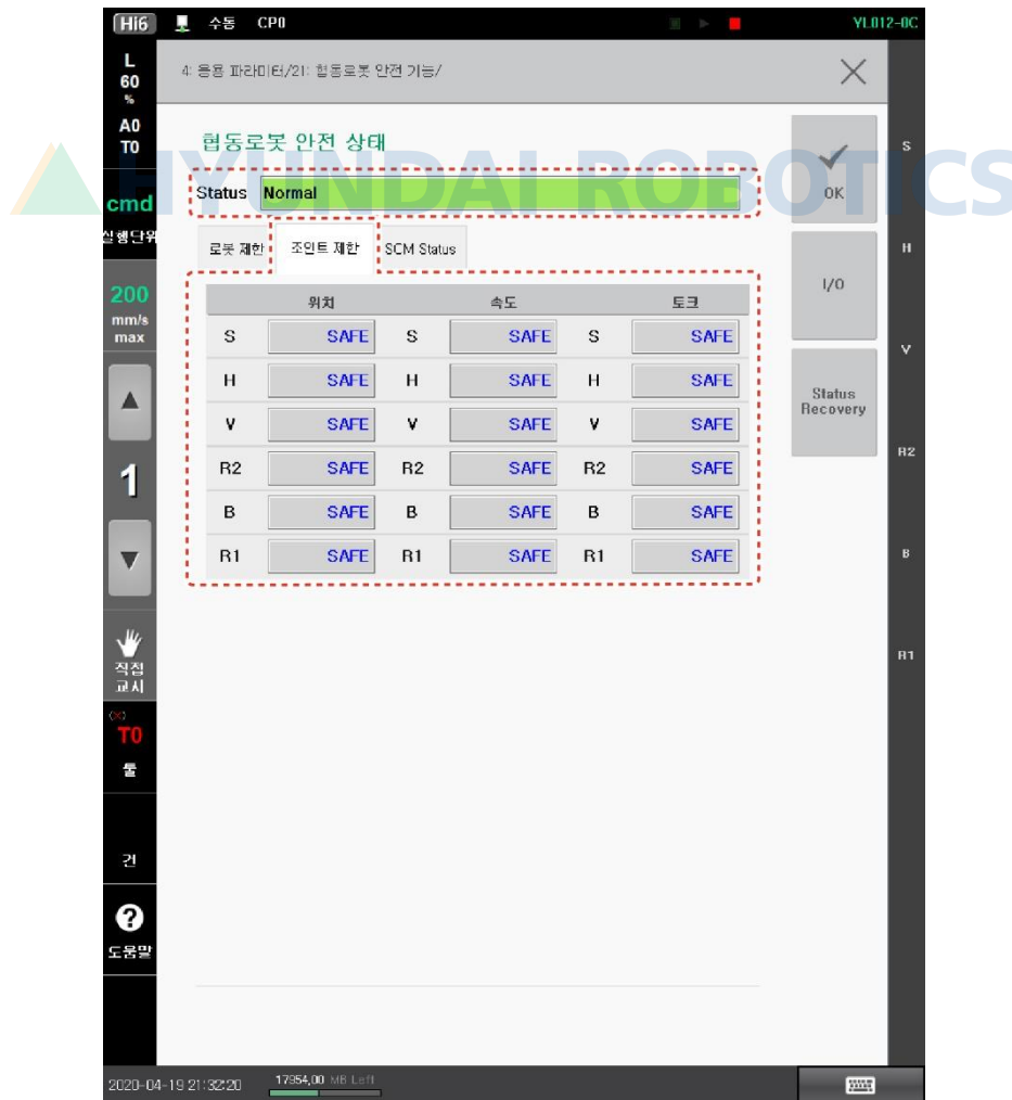
Figure 11 Safety conditions of collaborative robot: Joint restriction
